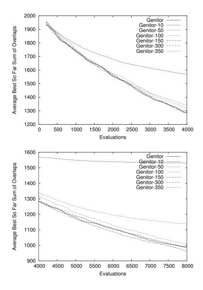
Figure 5: Evolutions of the average best value obtained by *Genitor* and its versions with a fixed number of selected positions for crossover. during 8000 evaluations, over 30 runs. The graphs were obtained for R1; best solution value is 773.
