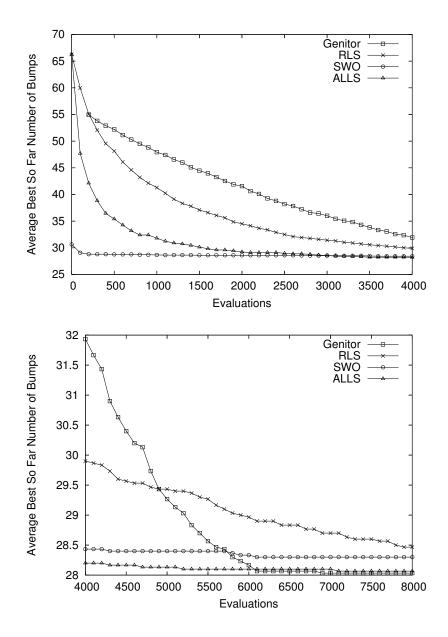
Figure 6: Evolutions of the average best value obtained by *Genitor*, RLS, SWO and *ALLS* during 8000 evaluations, over 30 runs. The improvement over the first 4000 evaluations is shown in the top figure. The last 4000 evaluations are depicted in the bottom figure; note that the scale is different on the y-axis. The graphs were obtained for R4; best solution value is 28.
