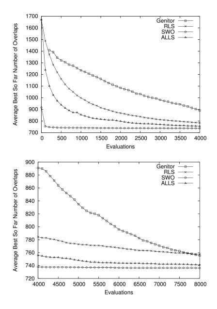
Figure 7: Evolutions of the average best value obtained by *Genitor*, RLS, SWO and *ALLS* during 8000 evaluations, over 30 runs. The improvement over the first 4000 evaluations is shown in the top figure. The last 4000 evaluations are depicted in the bottom figure; note that the scale is different on the y-axis. The graphs were obtained for R4; best solution value is 725.
