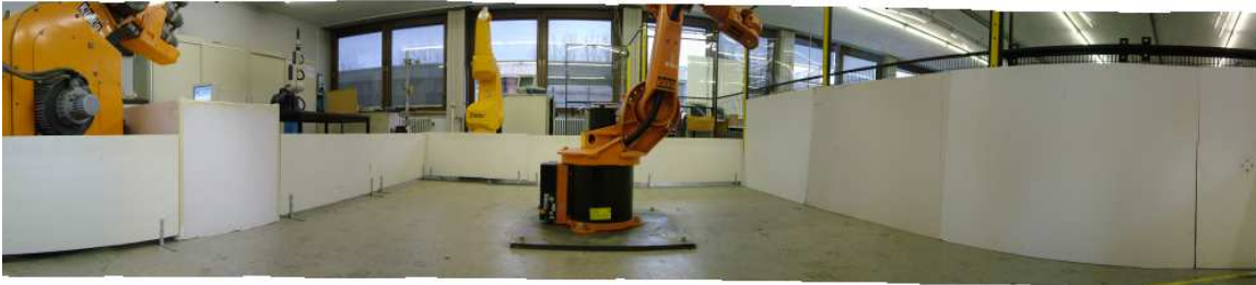
Figure 16: Panorama taken from the Sick LMS 200 range finder mounted on a Kuka 361 industrial robot. The environment consists of a rectangular ‘room’ with an object (a Kuka KR 15/2 robot) in the middle. We show that even for this simple static environment, the presented sample-based full scan model outperforms the Gaussian-based state of the art models.
