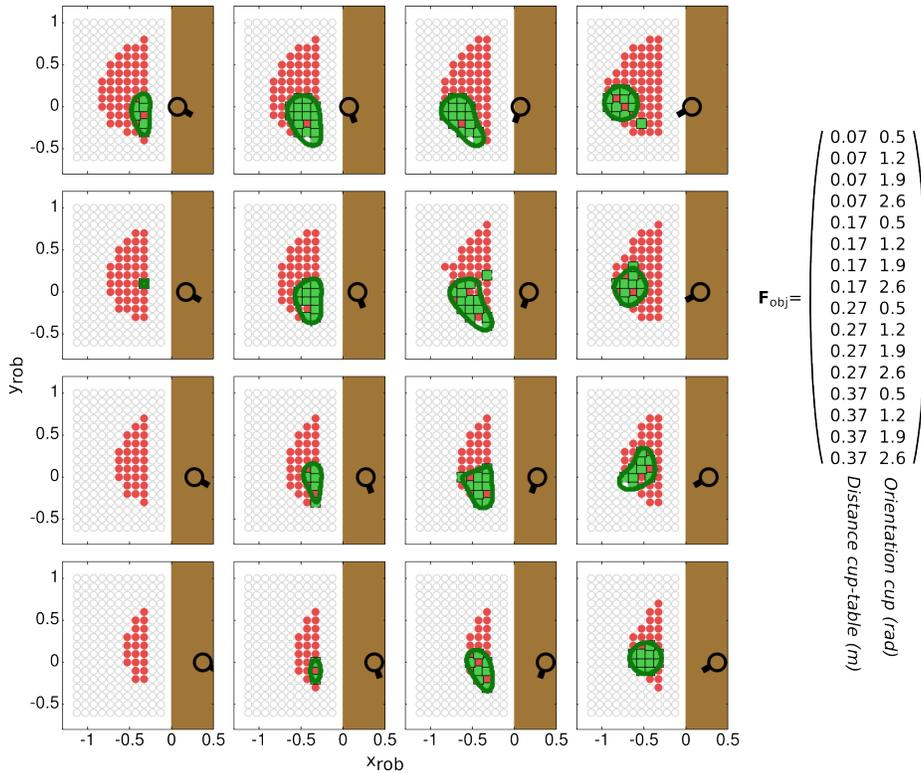
Figure 6: Results of data acquisition for 16 target object poses, listed in the matrix  $\mathbf{F}^{obj}$ . Markers correspond to the center of the robot base. Green squares and red circles represent successful and failed grasps respectively. Bright circles were not executed as a successful grasp is deemed theoretically impossible by capability maps. The dark green hulls are the classification boundaries (Section 3.2).
