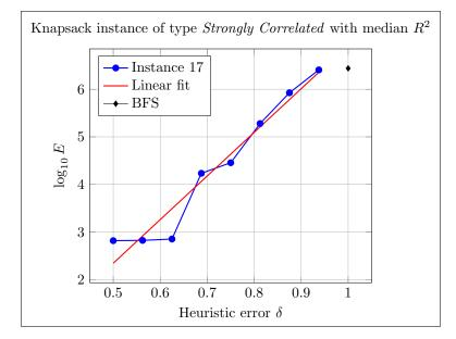
Figure 3: Graph of  $\log_{10} E$  and its least-squares linear fit for the Knapsack instance of type Strongly Correlated with the median  $R^2$  (see data in Table 3).
