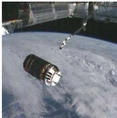
Figure 23: H-II Transfer Vehicle (HTV), a Japanese unmanned cargo vehicle, conducts autonomous rendezvous with the International Space Station. Image courtesy of NASA.
