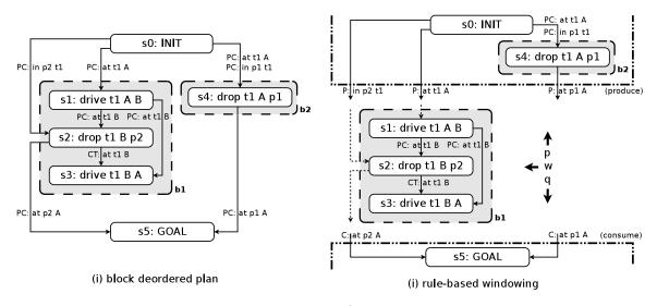
Figure 15: Window formation by applying the 1<sup>st</sup> rule of the rule-based windowing heuristic over block b1, i.e.,  $w \leftarrow \{b1\}, p \leftarrow Un(b1)$ . The unordered block b2 is placed in its predecessor set. Note that this window can be optimised by removing s3 because this step has no causal link to its successors.
