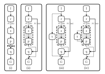
Figure 8: Formation of a block  $\{s,p\}$  and addition of a causal link  $\langle r,m,q \rangle$  in (ii) in order to remove the reason PC(m) behind the basic ordering constraint  $p \prec q$  from (i). Different situations, (iii and iv), where a threat, t, may be active to  $\langle r,m,q \rangle$ .
