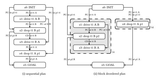
Figure 6: A sequential plan and a block deordering of this plan with two unordered blocks b1 and b2. Ordering constraints are labelled with their reasons: producer–consumer (PC), i.e., causal link, deleter–producer (DP), and consumer–deleter (CD). Note that no ordering constraint in the sequential plan can be removed without invalidating it. Thus, step-wise deordering of this plan is not possible.
