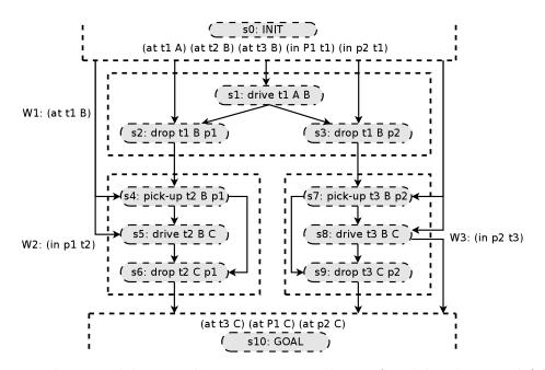
Figure 17: Three candidate windows, W1, W2, and W3, found by the causal followers windowing heuristic for atoms (at t1 B), (in p1 t2), and (in p2 t3) respectively. None of them are improvable. However, the composite window formed by merging W1 and W2 is improvable by substituting the delivery of package p1 (from location B to C) provided by truck t2 with truck t1. This is because the atom (at t2 C) is not required by any of its successors (i.e., the goal in this example).
