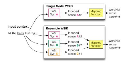
Figure 1: A comparison of the single-model and ensemble WSID systems, showing how the ensemble combines the output of multiple WSI models using a single mapping function.
