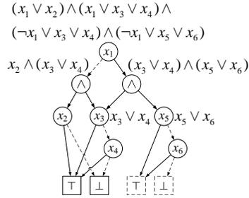
Figure 8: Example on how COMPILER runs, where  $\mathcal{C}$  is depicted in Figure 2a. After  $x_1$  is assigned *true*, we decompose the resulting formula into two parts, and detect that  $x_3 \vee x_4$  has been compiled; and thus we reuse the previous result
