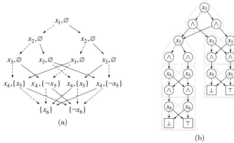
Figure 4: An ROBDD- $L_\infty$  (a) over chain in Figure 2a, and an AOBDD (b) over tree in Figure 2b, where each meta-node is depicted by a dash box
