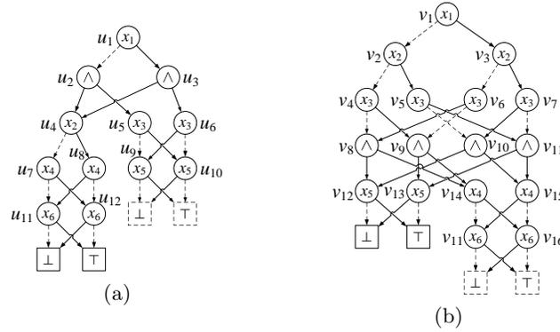
Figure 3: An  $\text{ROBDD}[\wedge_2]C$  (a) and an  $\text{ROBDD}[\wedge_1]C$  (b), where  $C$  is depicted in Figure 2a
