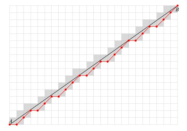
Figure 3: If A has line of sight to B then  $\lfloor AB \rfloor$  is a path from A to B.
