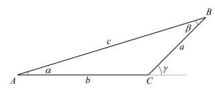
Figure 2: Proof of Lemma 4: For any fixed  $\gamma$ , the relative (percentage) difference between a + b and c is maximized when a = b.
