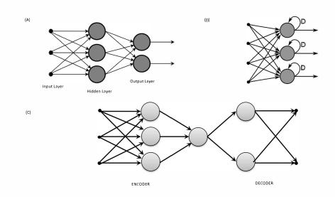
Figure 1: Feed-forward Neural Network (A); Recurrent Neural Network (B) and Encoder-Decoder (C) schemas.
