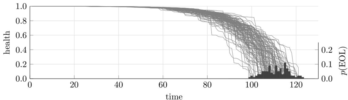
Figure 3: An EOL prediction illustration, with an overlay showing the  $p(\text{EOL})$  distribution
