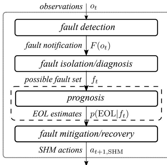
Figure 2: A typical contemporary SHM architecture
