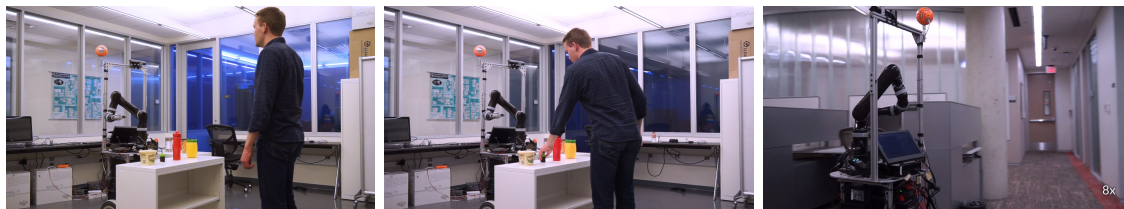
(a) The human says to move a rattling container from one room to another. (b) The robot asks questions about local items to learn a new rattling property. (c) The robot autonomously navigates to the specified location to search for the object.
