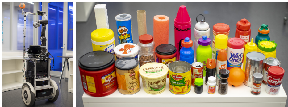
Figure 6: Left: The robot platform and arm used in our demonstration and for exploring objects. Right: The objects explored by the robot for grounding perceptual predicates.
