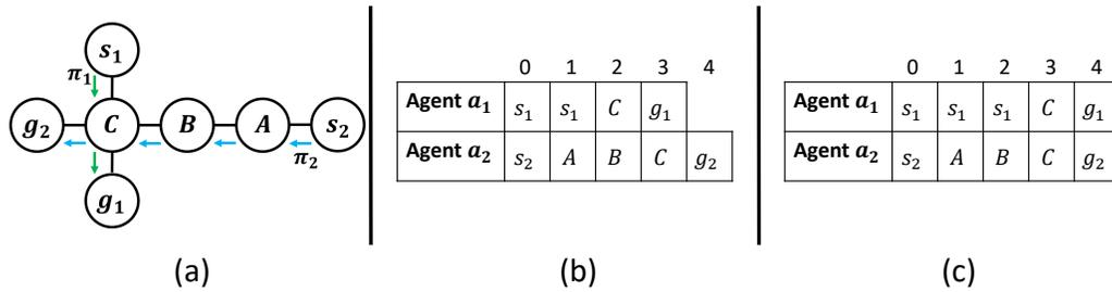
Figure 1: (a) A MAPF plan  $\pi$  (b) The planned execution of  $\pi$  at time 1, after agent  $a_1$  experienced a delay (c) The planned execution of  $\pi$  at time 2, after agent  $a_1$  experienced 2 delays.
