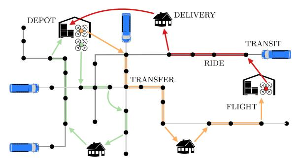
Figure 1: Our multi-drone delivery framework allocates delivery sequences to drones and plans routes for them to piggyback on public transit vehicles, while delivering packages from depots to the requested locations. Our framework is scalable and strives to minimize the *delivery time makespan*, i.e., the maximum delivery time for any individual package.
