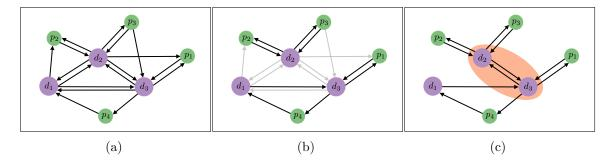
Figure 3: The MERGESPLITTOURS algorithm for delivery sequence allocation has three key steps: (a) The allocation graph is defined for the depots  $d_{1:3}$  and package destinations  $p_{1:4}$ . (b) The MCT step yields a solution that connects each package delivery with the depot from which the drone is dispatched and the depot to which it returns. (c) A tour merging steps merges the depots  $d_2$  and  $d_3$  into a single cluster, corresponding to line 10 of the algorithm.
