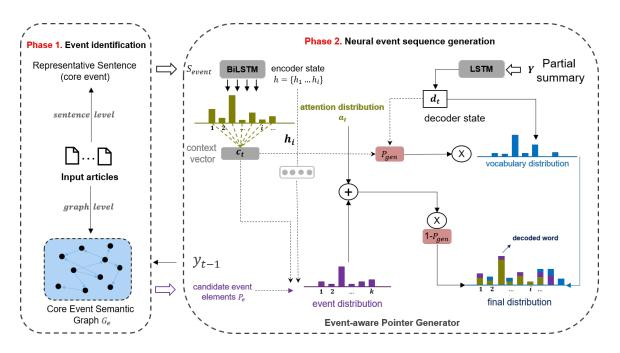
Figure 2: The overall architecture of our two-phase MES framework. At the event identification phase, input articles are fed into a graph-based extraction network for sentence-level and graph-level event detection. Then, at the generation phase, the extracted representative sentence  $S_{event}$  and event semantic graph  $G_e$  are further summarized in succinct event sequence through the proposed event-aware pointer generator.
