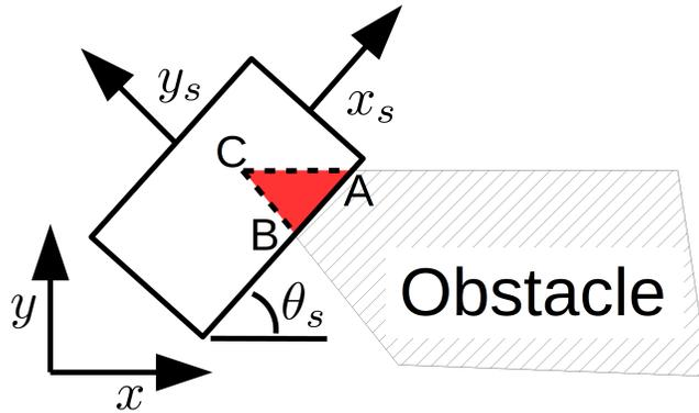
Figure 16: The intersecting region  $\mathcal{W}_{int}$  is the triangle defined by  $ABC$ . The dashed lines represent interface facets; they are used to compute the partial derivatives of the change in intersection area as a function of the decision variables.
