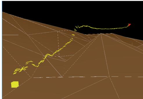
(b) A trajectory under larger uncertainty in the ocean currents. The trajectory optimizer generates a significantly different trajectory than the case with low uncertainty.
