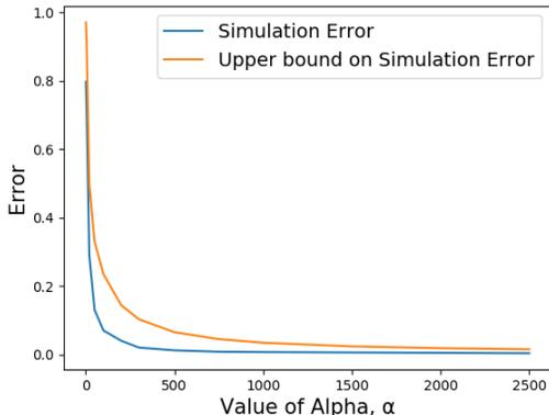
Figure 19: Comparison of the chance constraint error in simulation versus the upper bound on error, Eq. (67). The error is for a single trajectory knot.
