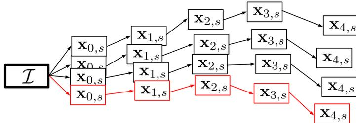
Figure 21: Illustration of the trajectory sampling and simulation strategy used by SMMC. The red trajectory is in collision and its  $\mathcal{W}_{int,s}$  is positive.
