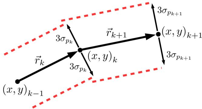
Figure 10: Illustration of the geometry used to validate a trajectory with respect to the chance constraint where the state distribution is assumed Gaussian. The trajectory is checked for collisions within three standard deviations on each side of the  $(x, y)$  states. In general,  $\sigma_p$  increases with each trajectory knot  $k$ .
