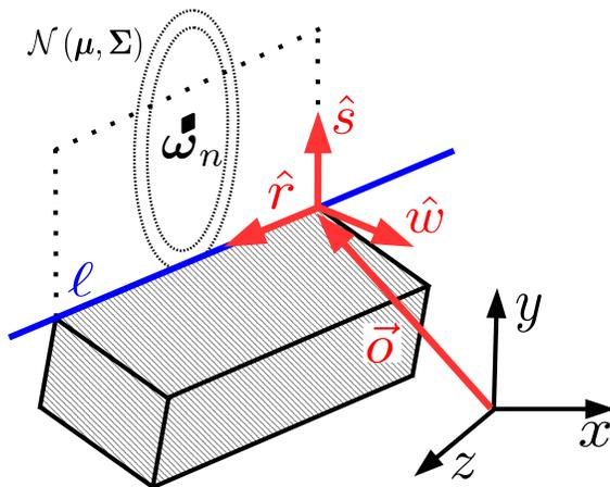
Figure 12: Illustration of the projection of the state distribution onto the landmark region for a 3D workspace. The dotted ellipses indicate the projection of the multivariate Gaussian onto the plane. The distribution is then integrated from the line  $\ell$ .
