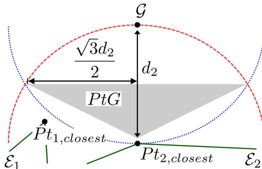
Figure 35: Geometry illustrating the width of the Polytope to Goal required for guaranteed termination. Similar geometry holds for a tetrahedron PtG in 3D.
