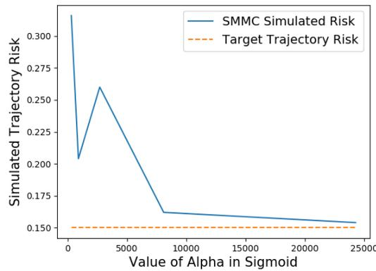
Figure 31: Plot depicting SMMC’s ability to approximate the chance constraint in simulation as a function of the sigmoid’s  $\alpha$  parameter
