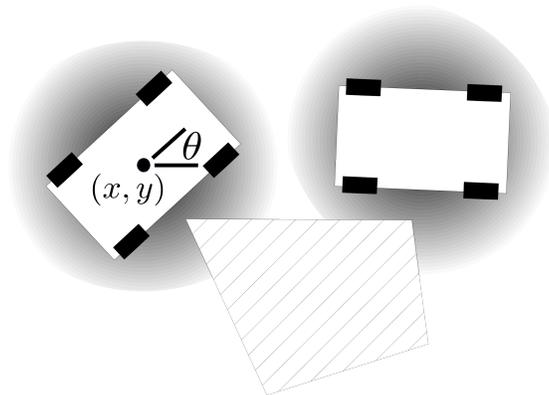
Figure 13: Computing the collision risk of even a simple rectangular shape is challenging. A possible distribution of the rectangular car’s state is shown in gray. Not only is there uncertainty in states  $(x, y)$  but also orientation  $\theta$ . An integration to compute the collision risk must be performed over all configurations that collide.
