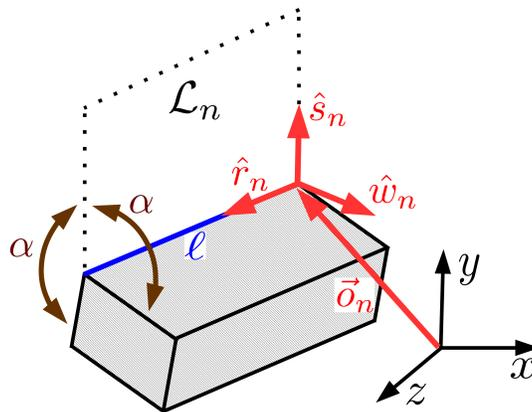
Figure 5: The plane and coordinate system that represent a landmark region  $\mathcal{L}_n$  for a 3D workspace. The dotted lines do not represent a constraint; they are shown to illustrate the plane.
