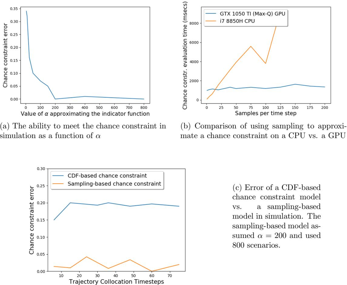
Figure 27: Numerical results of the sampling-based chance constraint model using collocation trajectory optimization
