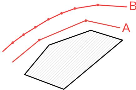
Figure 34: Illustration of how trajectories can become more conservative simply by decreasing time step size when the stochastic process variance is held constant. The diagram assumes the probability of failure is evaluated only at trajectory knots (red dots). For the same variance, trajectory A has fewer waypoints (a larger time step) and therefore fewer evaluations of path risk. This enables the optimizer to bring it closer to the obstacle while maintaining the overall chance constraint.
