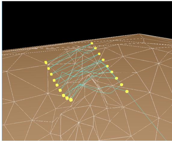
Figure 25: Illustration of the lawnmower motion primitive where the glider explores the ridge at the caldera’s northeast corner. The trajectory is denoted by cyan lines with lawn mower goals in yellow.
