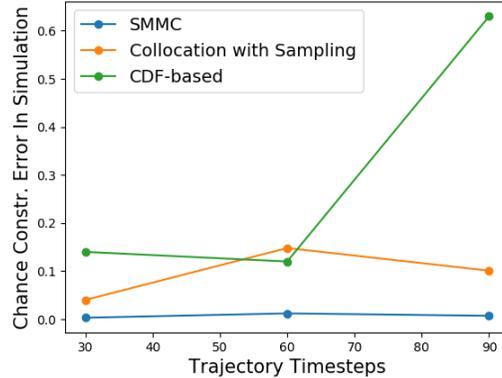
Figure 30: Comparison of the three chance constraint models’ ability to approximate the chance constraint in simulation for the Dubins car
