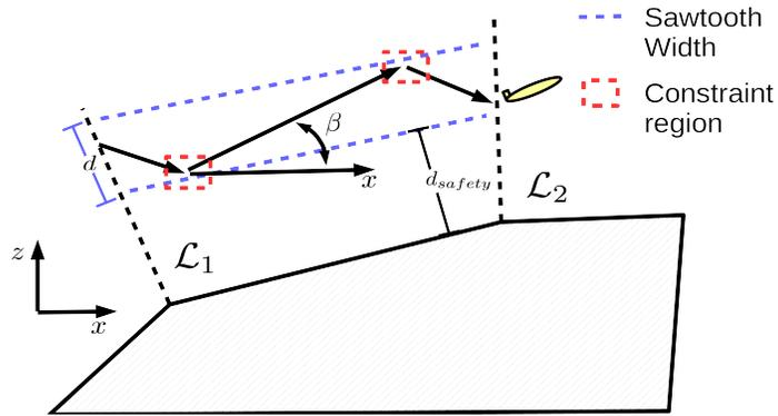
Figure 24: Integrating the glider’s sawtooth trajectory with the region planner’s  $\mathcal{L}$ . The glider travels at an angle  $\beta$  to the horizontal in depth band  $d$ .
