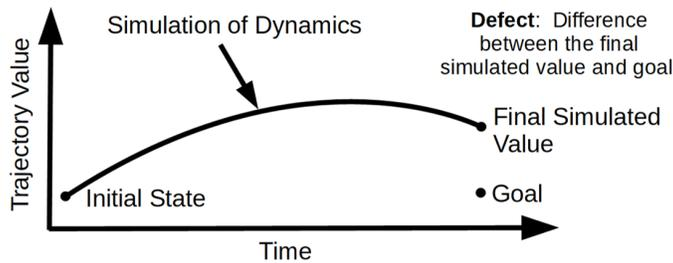
Figure 20: An illustration of the shooting method where a set of control inputs is simulated forward in time.
