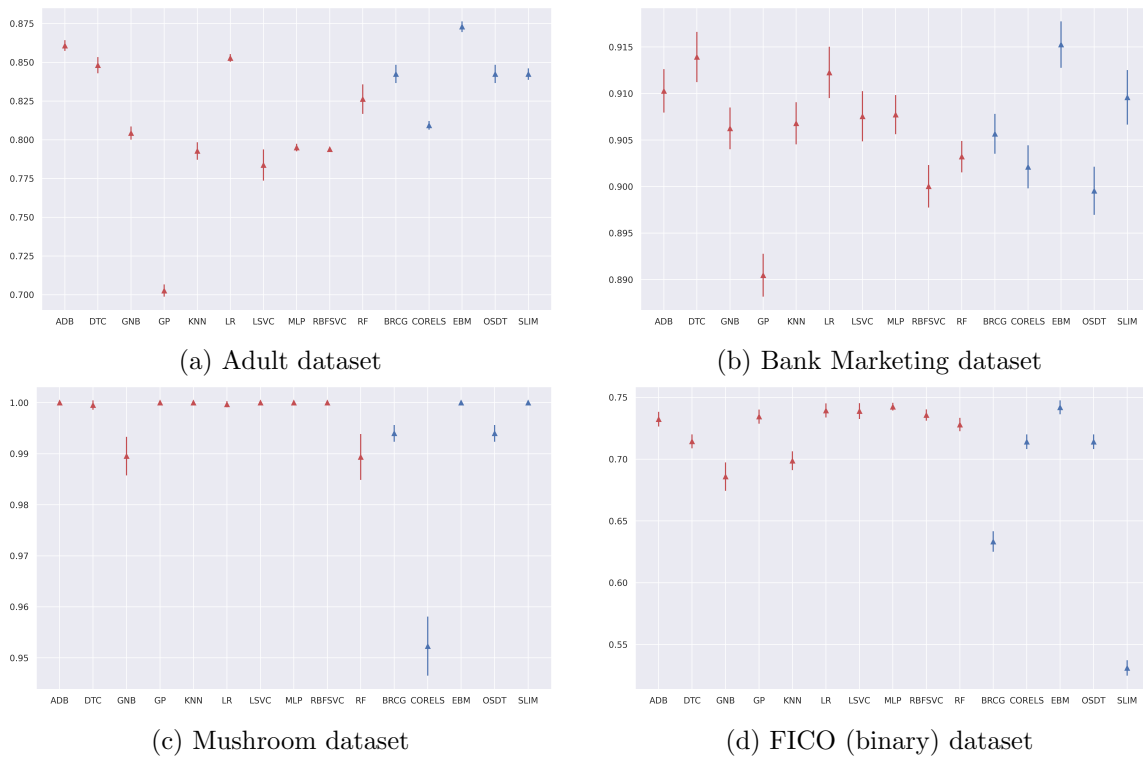
Figure 2: The CV accuracy of 10 standard box models (red, 10 leftmost models along the X-axis) and five interpretable models (blue, five rightmost models along the X-axis). The intervals represent the mean \pm one standard deviation.
