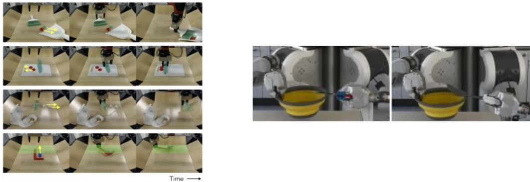
Figure 16: Examples of action modification in CPS: Action babbling through repeated interactions with the tool and object (Xie et al., 2019) (left), and action modification that adapts known tool use trajectories to new target objects, e.g., from a knife to a spatula (Gajewski et al., 2019) (right).
