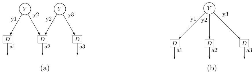
Figure 5: Example of wildcard matching for merging observation nodes. (a) On the left, the two observation nodes have zero-probability branches that are not shown. (b) In the equivalent strategy graph on the right, the two observation nodes are merged.
