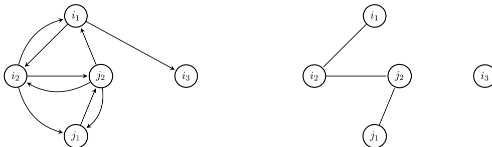
Figure 1: Left : a pool of patient-donor pairs, where an arc from a pair i = (p, d) to a pair j = (p', d') indicates that donor d is compatible with patient p' . Right : the corresponding compatibility graph.
