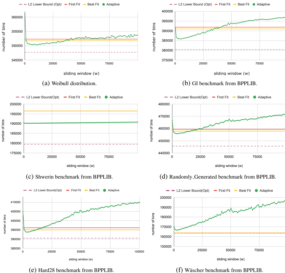
Figure 6: Number of opened bins for sequences from an evolving distribution. Note that, for the Shwerin benchmark, FIRSTFIT and BESTFIT open a similar number of bins and they practically coincide in the plot.
