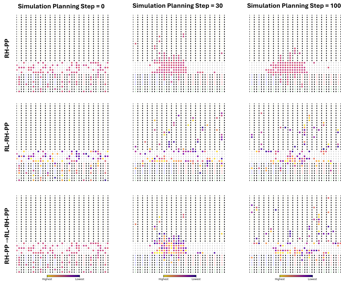
Fig. 19. Priority heatmaps for three planning methods (rows) at different steps (columns): 0, 30, and 100, as shown in Figure 18. Agents are shown in dots. The top row shows RH-PP, which assigns uniformly random priorities and experiences severe congestion by step 100. The middle row shows RL-RH-PP, which adaptively assigns higher priorities for agents in congested regions, sustaining high throughput. The bottom row shows switching from RH-PP (planning steps 0–29) to RL-RH-PP at step 30, effectively resolving inherited congestion by step 100. Lighter colors indicate higher priority assignments.
